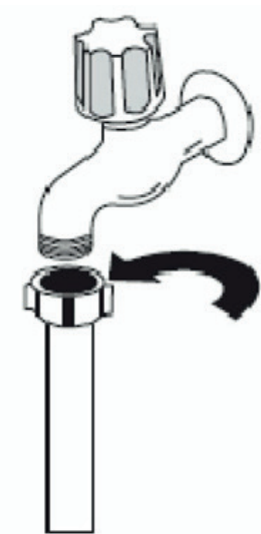
Figure 5: Connecting the supply hose to a \frac{3}{4} inch tap.
